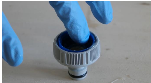
Tap nut adaptor with bottle cap glued in
