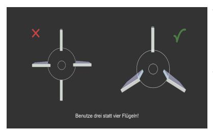
The fins are essential to ensure a stable flight of the rocket. Of course, they should be as light as possible, so choose a material which is very light but durable at the same time - like Corflute, for example. The fins of the rocket shouldn't be too large, because that usually results
