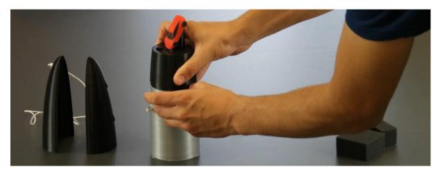
Wrap the rubber band around the two fairings and hook it into the tommy timer. This step works the same as on the Phoenix 3D parachute system. Now you can wind up the timer and use the trigger to hold it in place until launch.
