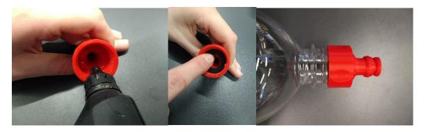
Mount the O-ring seal. Always check the nozzle for leaks in a safe environment before use. Go beyond the planned operating pressure during testing. Wear safety goggles and hearing protection.
