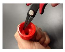
Fill the inner bottom with hot glue and insert the sealing ring. Then screw the nozzle onto a bottle and wait until the hot glue dries. The hot glue residues can now be removed.
