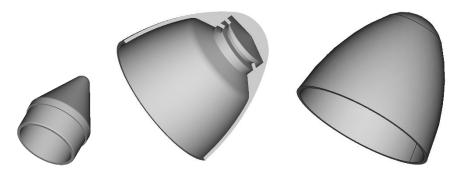
A 3D printer is ideal to print nosecones with low drag for water rockets.
